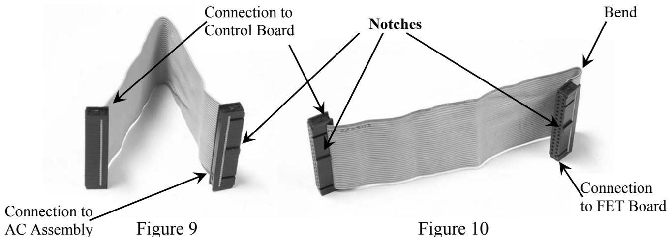
Install the ribbon cables between the boards following the connection instructions in Figures 9 & 10. After making the “Connection to the FET
